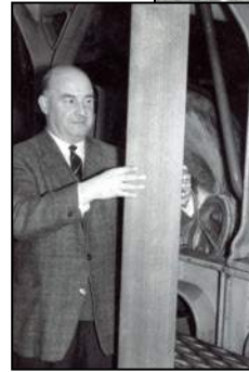
A QEII multiple crown watermark dandy roll on and off of the paper making machine. Photo taken by Harrison in the 1960s.
