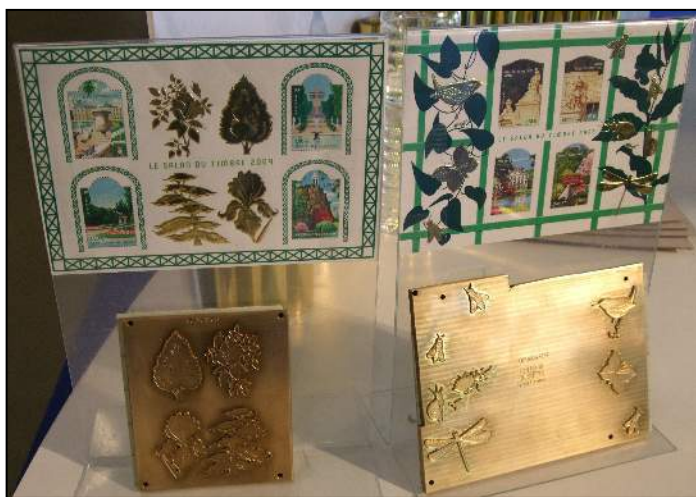
Brass male dies with MS above. Printed at ITVF France.
