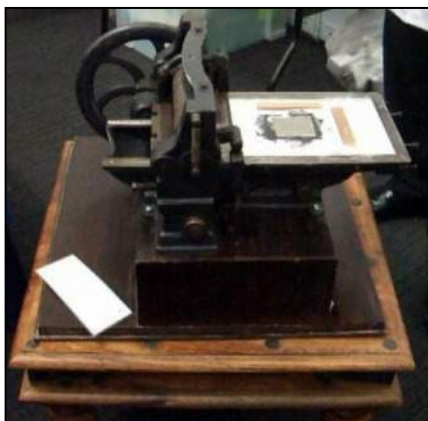
The die is in place on press bed.
